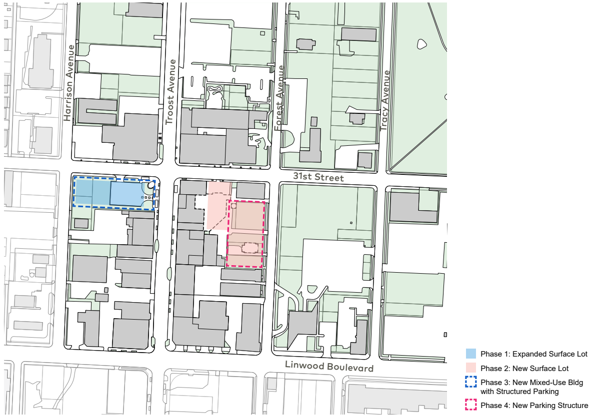
This diagram illustrates an intermediate phased parking scenario discussed by several developers in the area. Refer also to the strategy in the Implementation Playbook that references the need for a comprehensive shared parking plan, including phasing for immediate and future needs.
